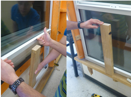
19. Carefully remove the prop and slowly lower sash. Note: Some downward force may need to be applied to disengage balances for the first cycle.
