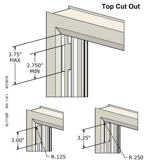
Maximum length of 3.75" for both the cut out and space above the cut out.
