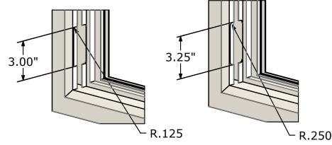
Maximum length of 4.75" for both the cut out and space below the cut out.
