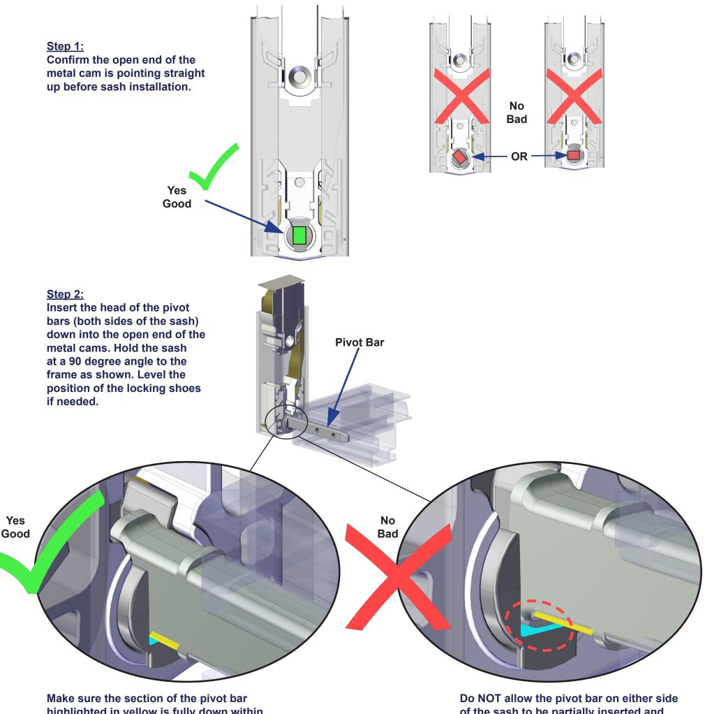
highlighted in yellow is fully down within the metal cam. The T head nubs of the pivot bar must be beyond the front lip of of the sash to be partially inserted and raised out of the metal cam when tilting the sash back into position. This can
