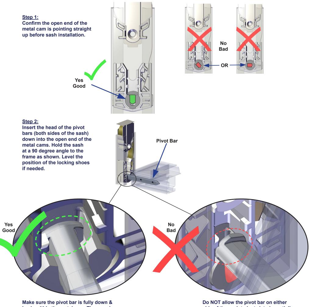
back, within the metal cam. The round head of the pivot bar must be beyond the front lip of the metal cam on both sides Do NOT allow the pivot bar on either side of the sash to be twisted, partially inserted or raised above the metal cam when tilting the sash back into
