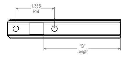
When ordering a special length the "B" dimension is required. Example, if "B" = 2.47" then order 211-2.47
