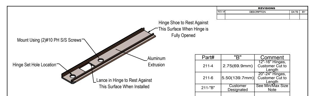
211-"B" In Hinge Limit Device for Projection hinges
